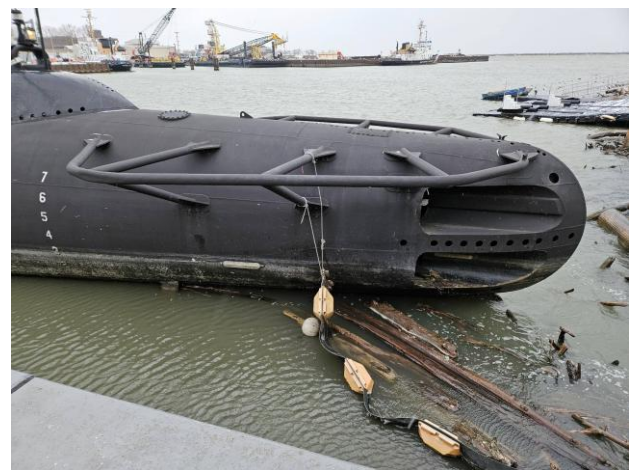
Cleveland; Strong easterly winds created more seiche conditions and dropped the water levels more than they were a few weeks ago. USS Cod curator Ben Yanke documented the exposed rudder and stern features in this image. More of Cod's hull bottom sits on the uneven lake bed, resulting in a rare 2 deg. starboard list until water levels rise again. JRSC fb pg; Gerald Gates 12-22-25
