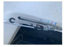
Position of marks for accelerating out of a tac. Then, once the boat is flat and at full speed I ask crew to Go to "full trim" or "trim to mark."
