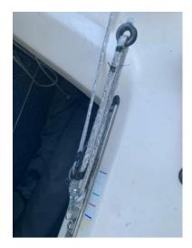
Also notice that I have colored marks (could use a scale here) for jib car location. My two most common settings are "Go Green" & "Go White" (I can't ever remember saying "Go Blue", but Hey, I'm a Spartan fan!). Crew can communicate easily the car position and quickly adjust as requested. (Tip: if the wave angle to bow is different on each tac, consider lead forward a hole on the tac for direct waves.)
