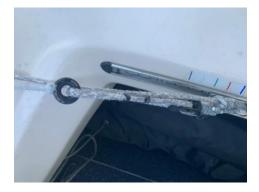
Big power up setting for after slamming into a wave during a tac or just a casual cruise. Note: I use a "friction ring" (actually, low friction) in place of blocks on a tail for my 2:1 jib lead.
