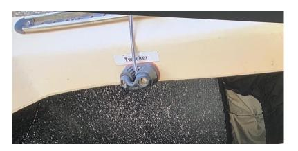
Using them is simple. "Full on" or "completely released." Instead of putting the guy in the hook trim full on. Instead of releasing from guy hook release the twing from cleat. SIMPLE! Plus, no-one has to reach outside of the boat to snag a spinnaker guy. Just pull in the twing from in the cockpit. Heck, even the skipper can reach forward and do it if needed. EASY ©
