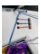
Placement of twing cleat inside cockpit across from side-stay (more on this below)
