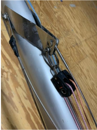
mast "hounds" with dual sheave
