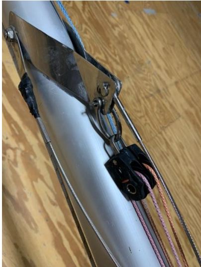
mast "hounds" with dual sheave
