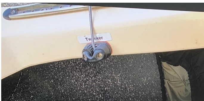
Below: Placement of twing cleat inside cockpit across from side-stay (more on this below). When sailing, that thin twing line just hangs down.
