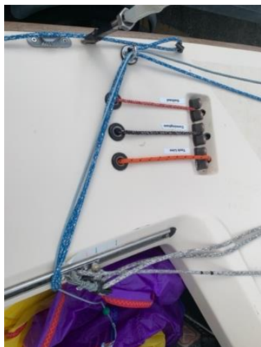
Left: Guy hook primarily used to organize spin sheet/halyard.
