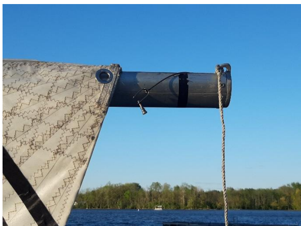
Figure 2 - Outhaul Disaster Preventer – an 18" piece of 1/8 line
