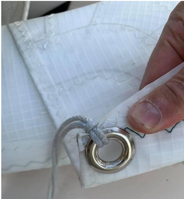
Pig tails attached to jib clew. This actually holds! Or you can tie blocks directly to clew.
