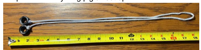
My jib pig tail lead. 3mm Spectra w 10mm lead rings
