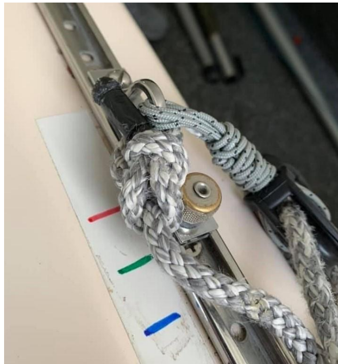
Tie off end jib sheet to base of jib car or to becket on jib car block when using 2:1 system
