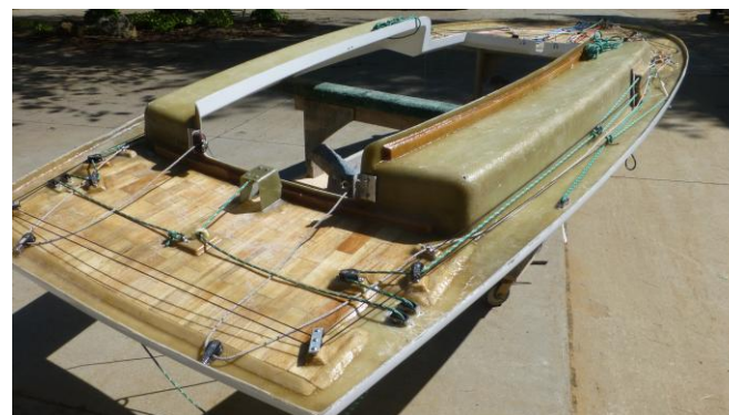
Aft (above) and forward (below) underside rigging on a new Interlake deck
