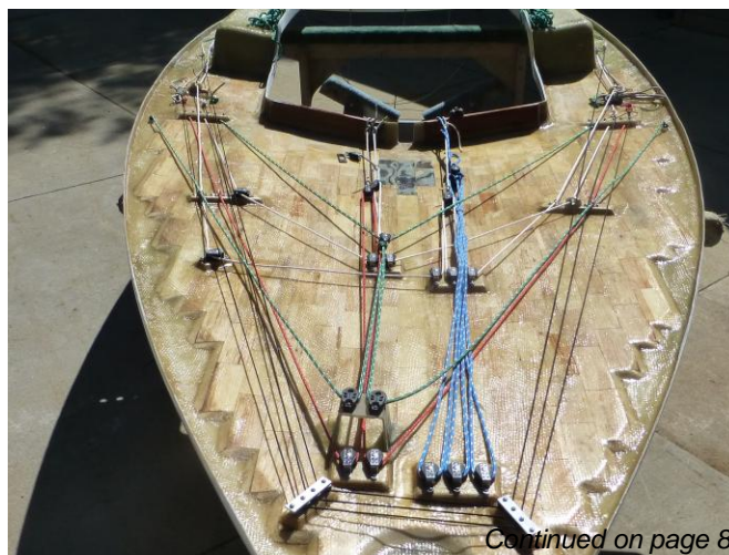
Aft (above) and forward (below) underside rigging on a new Interlake deck
