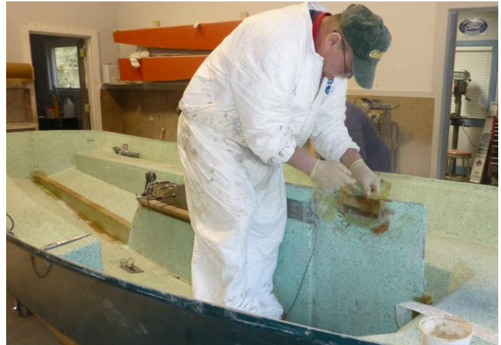
Mike Plodzick modifies an existing hull to accept new hardware
