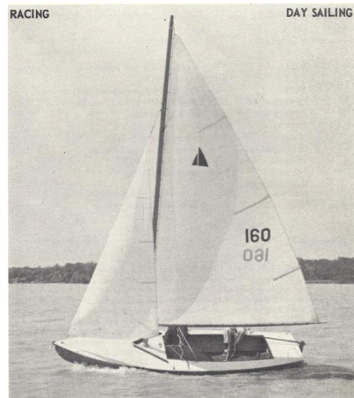
While Interlake 160's hull was Fiberglas, the deck was wood. Boat 161 was the first boat with a Fiberglas deck.
