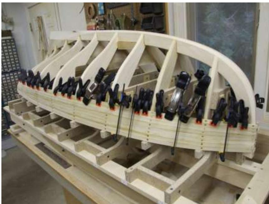
So, Dave telephoned Gartside in British Columbia, and he agreed to forward a set of study plans, considering the 1"=1'-0" (1/12<sup>th</sup> scale). Then they were developed on the computer, (lofted, if you will) and a table of offsets were calculated. From there, cross sections were drawn at each of the 10 main stations where the frames were to be located, and a set of scale templates were made from them. After that it was an easy task to have them printed and transfer the templates to wood.
